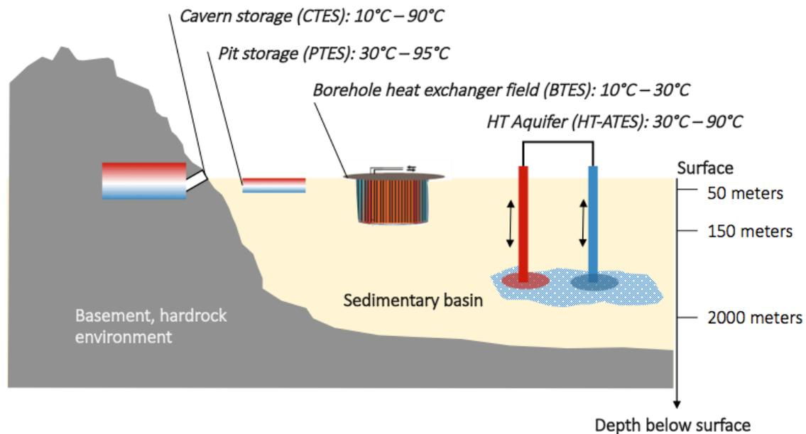
Fig. 2. Overview of the different UTES concepts regarding their position in an overall geological context. The graph also shows the depth and temperature interval of each application [Gregor Goetzl, personal communication].
