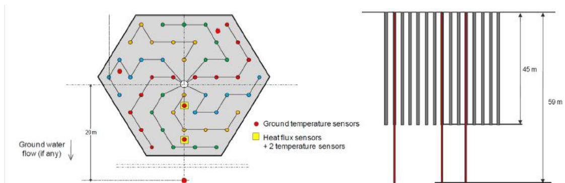
*Fig. 5. Sketch of the BTES system at Braedstorp, Denmark.*
