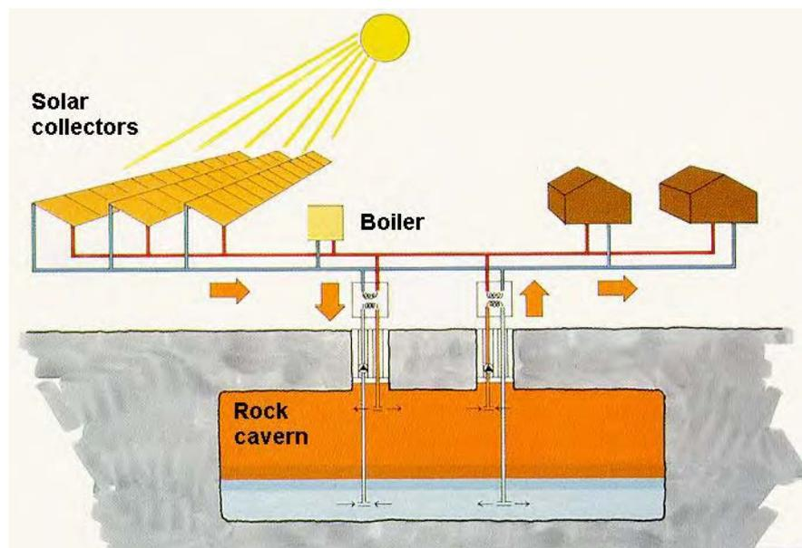
*Fig. 8 Sketch map of the integrated solar district heating system and CTES plant in Lyckebo, Sweden.*
