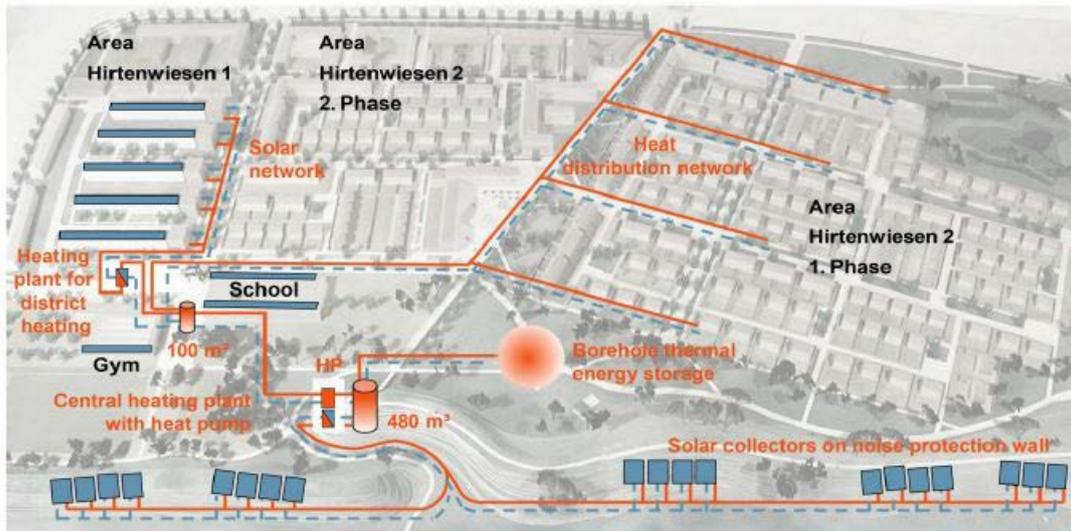
Fig. 6. Sketch of the solar district heating system in Crailsheim Hirtenwiesen equipped with a storage system made by water tanks and a BTES technology.
