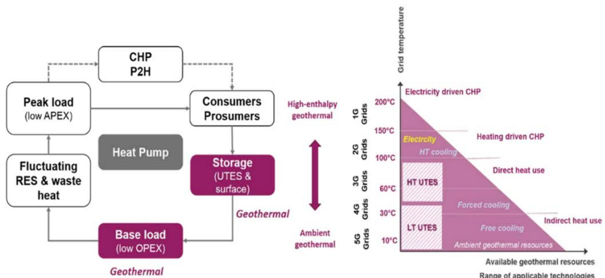
Fig. 1. Sketch of geothermal uses in district heating and cooling networks, from Goetzl et al. 2021.
