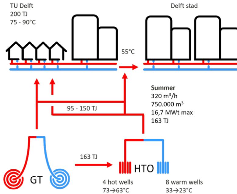
Fig. 3. HT-ATES example connected to the existing district heating network on TU Delft University, The Netherlands
